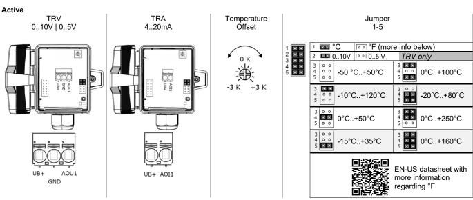
fig. (Measuring range and offset adjustment, default settings: +40 °C..+240 °F | 0 K)
