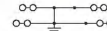
斜面双层八线接地端子 Double level angled type ground terminal block 8-wire
