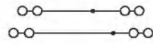
斜面双层八线接线端子 Double level angled type terminal block 8-wire
