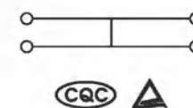
242系列两进两出带销钉侧面接线端子 242 Series 2-2 Feed Through Terminal Block With Snap-in Mounting Feet of Side-entry
