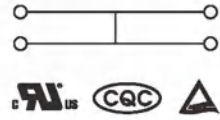
242系列两进两出侧面接线终端用端子 242 Series 2-2 Feed Through End Terminal Block With Snap-in Mounting Feet of Side-entry
